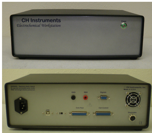
Front and rear view of the Model 400C, 600E, 700E, 800D, and 1100C series instruments
