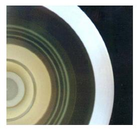
Three Bands of Particles During Sedimentation
