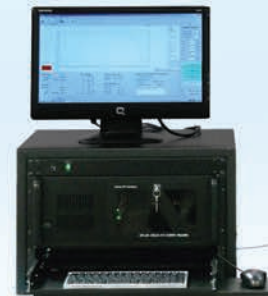
CT150 AAA Cell Tester Area of illumination 150 mm x 150 mm Shown with standard flat screen (touch Panel) Control Panel
