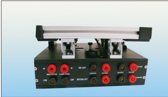
FIGURE 9: REAR VIEW OF THE FIXTURE- BANANA JACKS TO SELECT DIFFERENT CELL CONTACTING SCHEME
