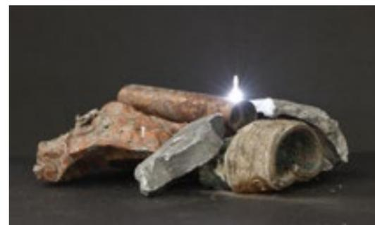
Classification of metals and alloys by means of laser-induced breakdown spectroscopy (LIBS) conducted with LIBSorter 300
