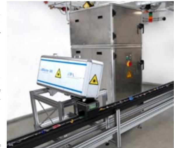
Mixed scrap metals that are transported on a conveyor belt for LIBS classification with LIBSorter 300 providing a rate of up to 25 pieces/s
