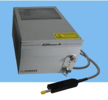
The EZRaman-N system features a narrow linewidth frequency stabilized laser, high throughput fiber optics probe, and an optically fast (f/1.6) spectrograph with TE cooled CCD detector. This system is easy to use with powerful and user-friendly RamanReader software, while providing excellent long term reliability with minimal maintenance.
