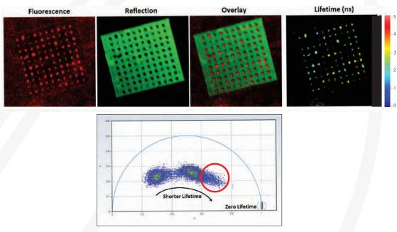
Fig 1- Phasor plots separate different lifetime species of Quantum Dots coated on the substrate, directly from the raw data. Ex. 470 nm, Em. 499-632 nm (Fluorescence), 475/35 nm (Reflection), scanning area 17.5µm x 17.5µm. (*Courtesy of Dr. Wenjie Liu and Dr. Yaowu Hu; Purdue University; West Lafayette, IN; USA*)
